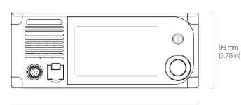
240 mm \*Flushmount cut out (9.44 in) 215 mm x 89 mm
