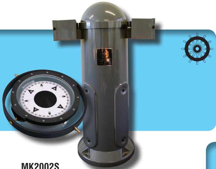
MK2002S Reduced height compass system according to current IMO legislation for vessels on restricted service or under 150 GRT. Approved by BV, CCS and Wheelmarked. Available either in reflector or non-reflector versions, in white or grey.
