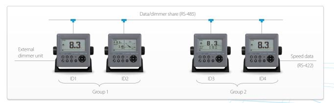
In this sample, the display with ID4 receives data (RS-422) from signal distributor and outputs vessel speed data (RS-485) to all connected display. Dimmer share has been separated in two groups, whereas group 1 can be operated by external dimmer and group 2 is linked pressing the button on the display.
