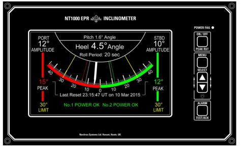
[The traditional mechanical "pendulum" type of heel measuring devices can provide reasonably accurate indications of angle, but this is largely confined to static situations whereas in a seaway, pendulum mass and inertia will invariably result in significant errors.
